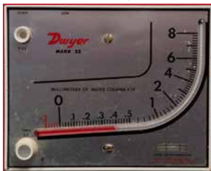
Figure 103: A manometer used to monitor air pressure within the house (the reading given is equivalent to 0.15 inches of water column).
