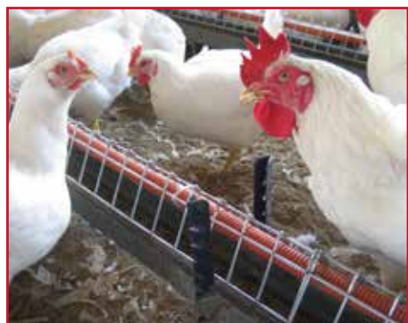
Figure 45: Separate-sex feeding system for females showing grills and the addition of plastic pipe in the apex.
