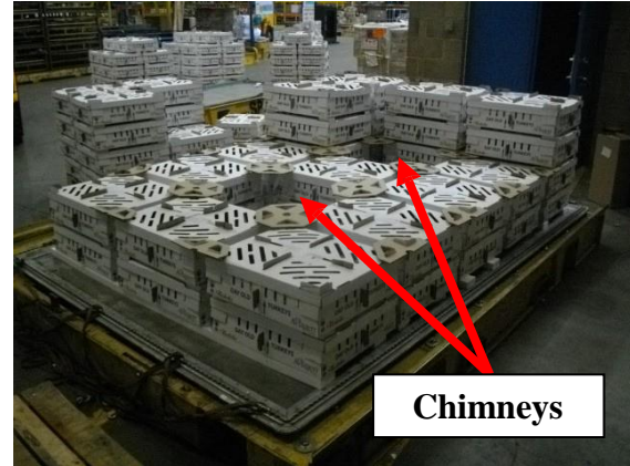
Built in chimneys
